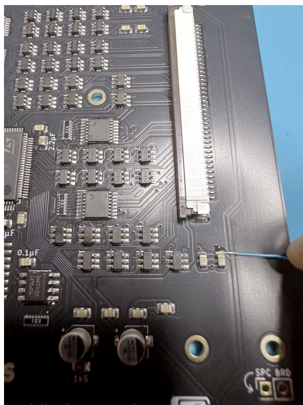
Apply flux and place the stripped end on the upper 5V capacitor pad.
