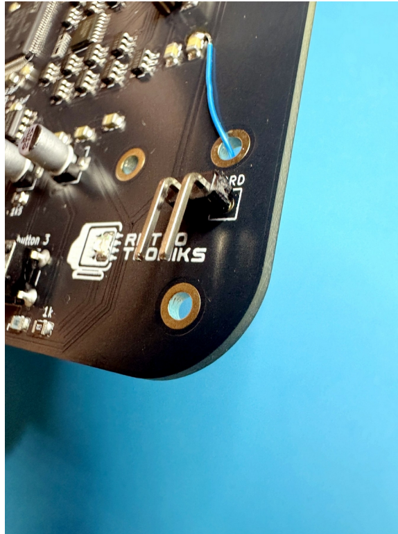
Recommended 90-degree header orientation.
