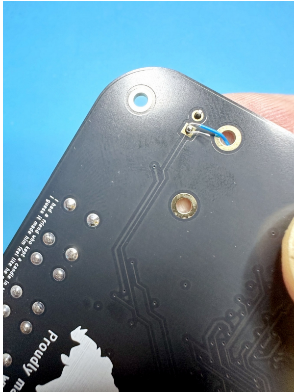
Wrap the wire around the square-pad 5V pin before soldering.
